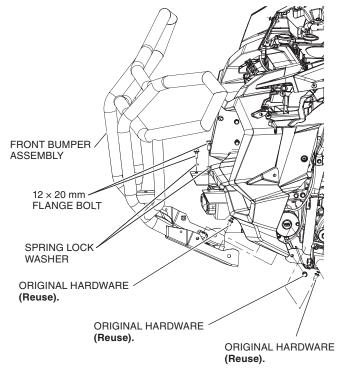
3. Tighten all the bolts to the values specified in the TORQUE CHART.
