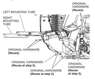
NOTE: If a winch will be installed, refer to the winch Installation Instructions, before continuing to Step 2.
